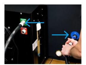
Tub Outlet to Chiller Motor Inlet:
