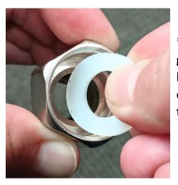
\*Hoses will have gaskets pre-installed, but please double-check before threading
