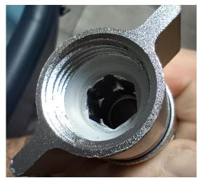
**Connect Hoses:** Hand Tight is acceptable, do not overtighten connections as this may strip the threads.
