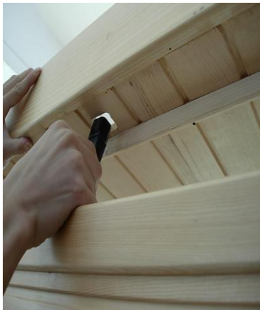
FIG-12 Slip cords/wires through corresponding holes
